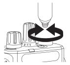
With the radio turned off, set the antenna in its receptacle and turn clockwise.
