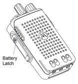
To remove the battery, turn the radio off. Move the battery latch into unlock position and hold.
