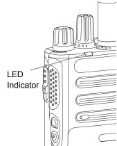
Solid yellow – Radio is monitoring a conventional channel or in Bluetooth Discoverable Mode. Also indicates fair battery charge when **Battery Strength** button is pressed.
