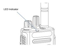
The LED lights up solid green while the radio is transmitting and blinks when the radio is receiving.
